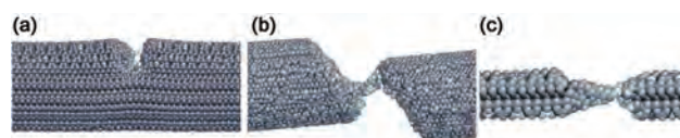
Figure 23. Snapshots of [110]-oriented Si NWs under tension in molecular dynamics simulations using the modified embedded atom method potential. Reproduced with permission. [266] Copyright 2007, Taylor&Francis. a) Brittle fracture of a 7-nm-diameter NW at 300 K. b) Ductile fracture of the same NW at 1000 K. c) Ductile fracture of a 2-nm diameter NW at temperatures as low as 100 K.
