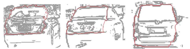
Fig. 8. Active contour detection. The red curves mark the detected contour of the corresponding vehicle.
