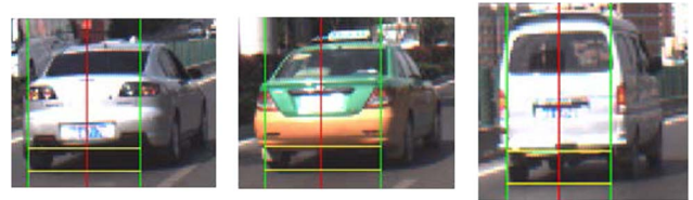
Fig. 7. Rectangular boundary detection. Three detection results with different kinds of vehicle are illustrated. The red lines mark the central position. The left and right blue lines mark the detected horizontal boundaries. The yellow lines mark the detected vertical boundary for the bottom shadow.
