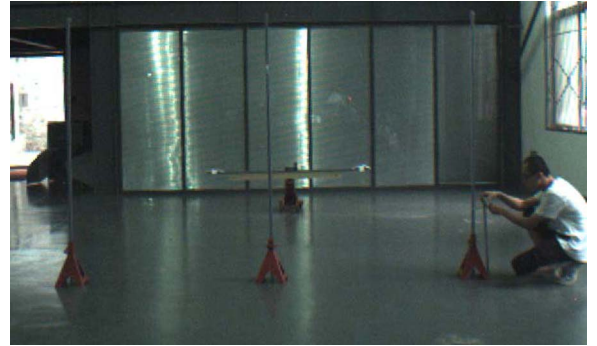
Fig. 2. Illustration of the spatial calibration process. The poles are regularly arranged and detected by the MMW radar and the monocular camera.
