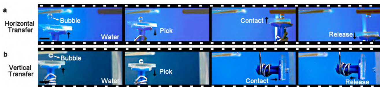
Fig. 5. The 80/240-patterned array SMP film is regarded as “mechanical hand” to realize bubble underwater transportation in horizontal direction (a) and vertical direction (b). The scale bars in (a) and (b) are 4.5 mm.
